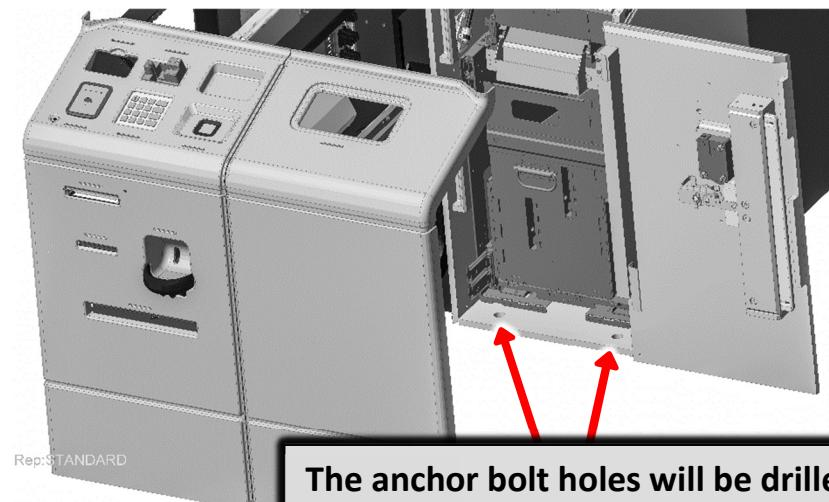
D. Use a hammer drill with an 18mm bit to drill through the anchor bolt mounting holes in the positions shown above. See figure at right for drill hole specifications.
