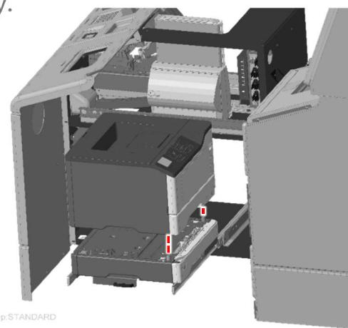
E. Plug in the AC power cord, USB Cable and ethernet cable that are located on the printer tray mount.
