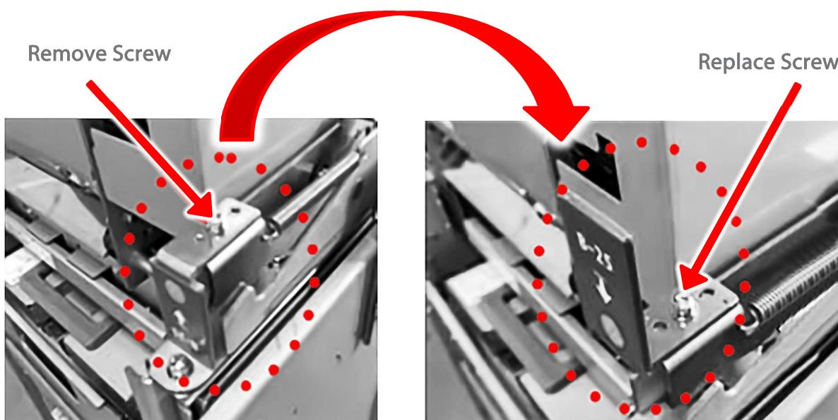
F. Move the retaining screw shown at right to the left-hand location.
