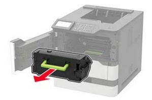
**3** Remove the used imaging unit.
