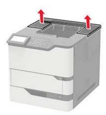
**5** Install the finisher on the printer.
