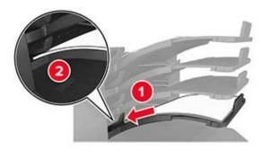
Note: If the paper is not under the bin arm, then a jam occurs due to an overfilled bin.
