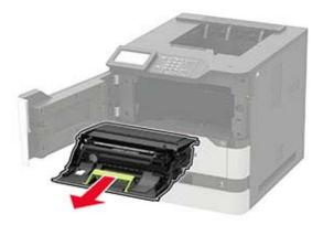
4 Remove the used transfer roller.
