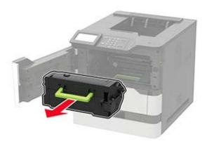
**3** Remove the used imaging unit.
