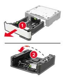
**5** Remove the used pick roller assembly.
