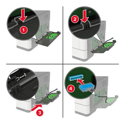
**a** Unplug the hard disk interface cable from the controller board.
