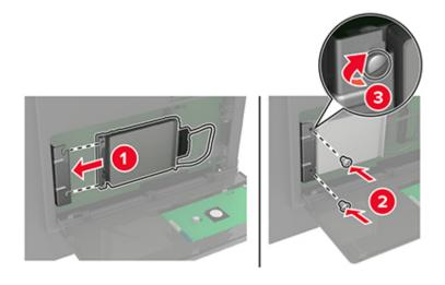
6 Attach the hard disk interface cable to the controller board.
