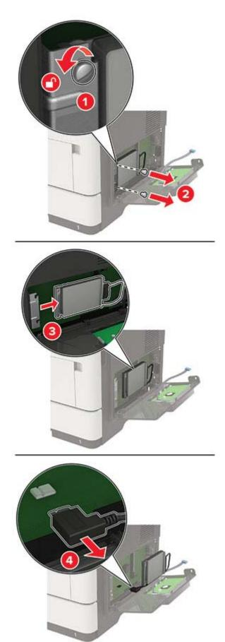
${\boldsymbol b}$  Connect the ISP extended cable to the ISP connector.
