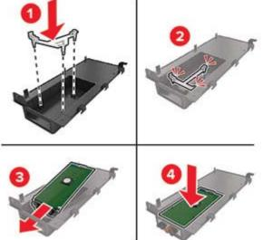
${\bf 5} \ \ {\rm Secure \ the \ ISP \ in \ place \ and \ attach \ the \ ISP \ extended \ cable.}$
