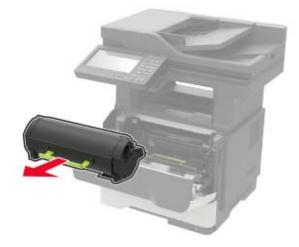
Remove the used imaging unit.
