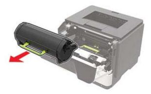
Remove the used imaging unit.
