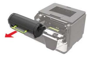
Remove the used imaging unit.
