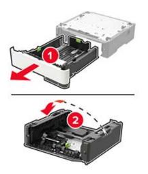
**5** Remove the used pick roller assembly.
