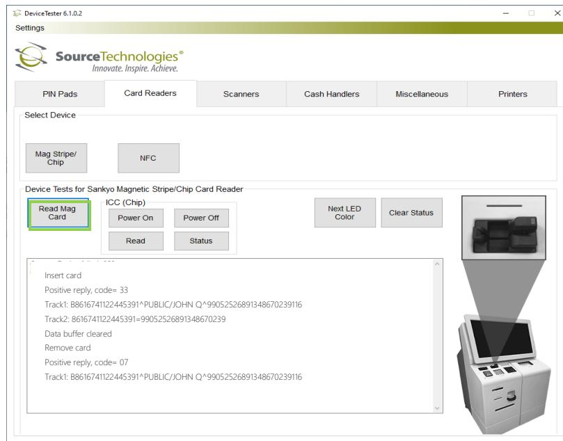
3. Tap the Power On button under ICC(Chip). Insert a card with a chip and tap the Read button.
