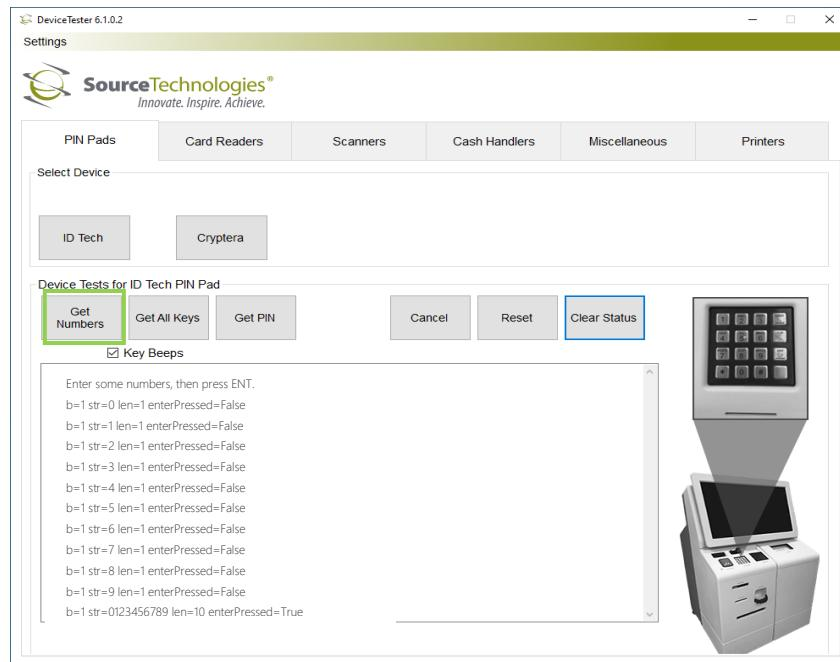
3. Tap the Get All Keys box to test operation of the \*, #, clear, blank keys followed by the enter key.
