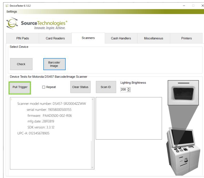
3. Lay the test card or ID card on top of the barcode scanner and tap the Scan ID. A snapshot of the image ID will show up in the lower right box.
