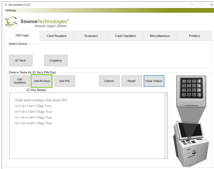
4. Tap the Get PIN box and enter any 4 numbers on the pin Pad followed by the enter key. Encrypted PIN should be displayed on the last line.
