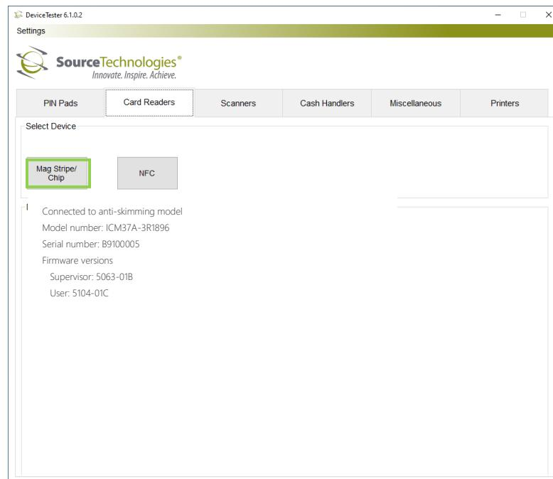
2. Tap the Read Mag Card button and insert and remove the card provided in the accessory kit. If done correctly you should get data with three track numbers.
