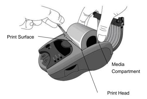
3. For media supply rolls with width less than 3 inches: Load media supply first, and then align the media roll to the right end for correct detection by the Media Sensor:
