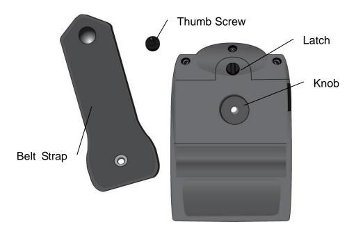
2. Attach the Belt Strap onto the Knob.
