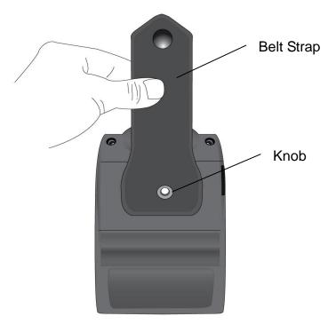
3. Insert the Thumb Screw onto the Knob, through the Belt Strap, and tighten clockwise until it is fully secured:
