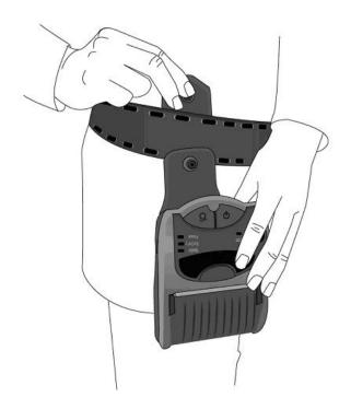
5. Pull down the top of the Belt Strap to attach the Snap:
