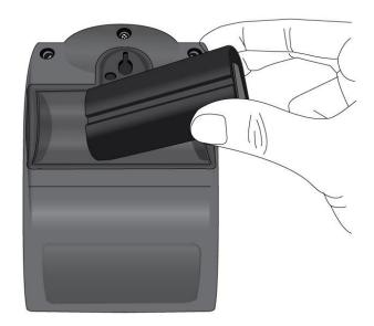
3. Replace the Battery Cover and rotate the Battery Cover Latch 90° to the left to lock in place:
