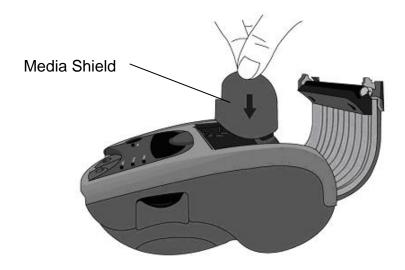
5. Pull a short length of media out of the printer. Close the Media Cover and press until you hear a click, to properly latch:
