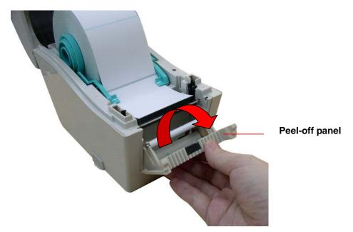
3. Lead the media through the backing paper opening, beneath the peel-off roller.
