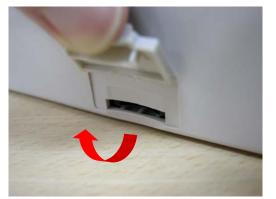
2. Insert the MicroSD card into the socket.
