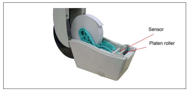
4. Place the media, printing side face up, through the media guides, over media sensor and place the label leading edge onto the platen roller.
