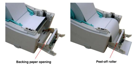
4. Push the peel-off panel back to the printer.
