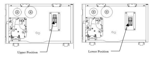
Figure 18 - Media Spindle Location
