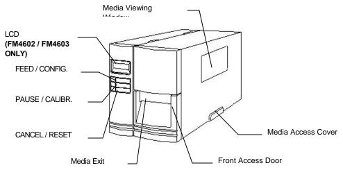
Figure 4 - Front and Side View
