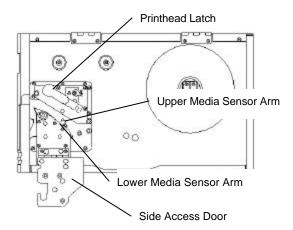
Figure 14 - Printhead Latch and Side Access Cover
