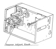
Figure 16 - Media Sensor Adjust Knob
