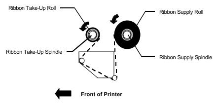
Figure 12 - Ribbon Routing
