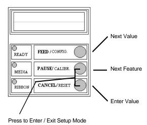
Figure 24 - Entering into Set-up Mode
