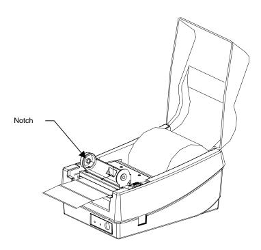
Figure 9 – Ribbon Holder Notch Location
