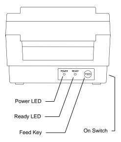
Figure 16 – Fastmark 400 Series Front Panel
