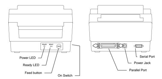
Figure 5 – Switches, Indicators and Connections
